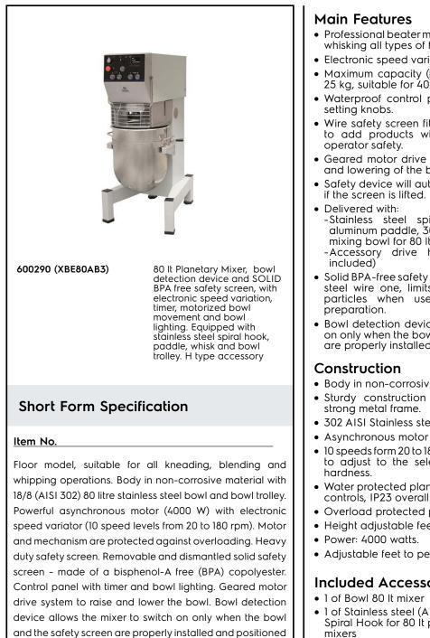
together. Equipped with accessory drive hub type H (accessories are not included). Supplied with 3 tools: stainless steel spiral kneading hook, cast aluminium paddle and stainless steel wire whisk.
